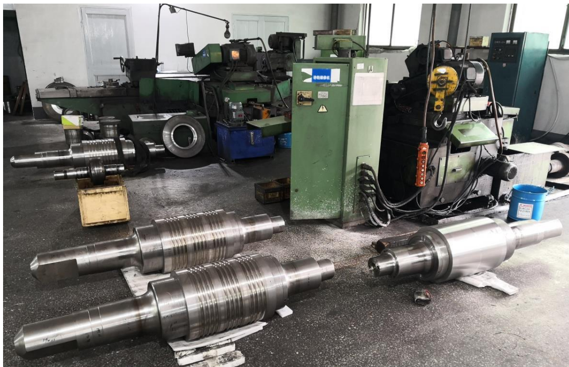
Composite roll finished processing workshop
